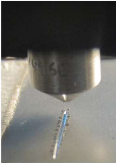
Stylus in Ducom scratch tester
