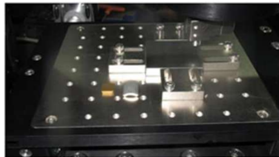
X - Y stage with sample holder for different size and geometry
