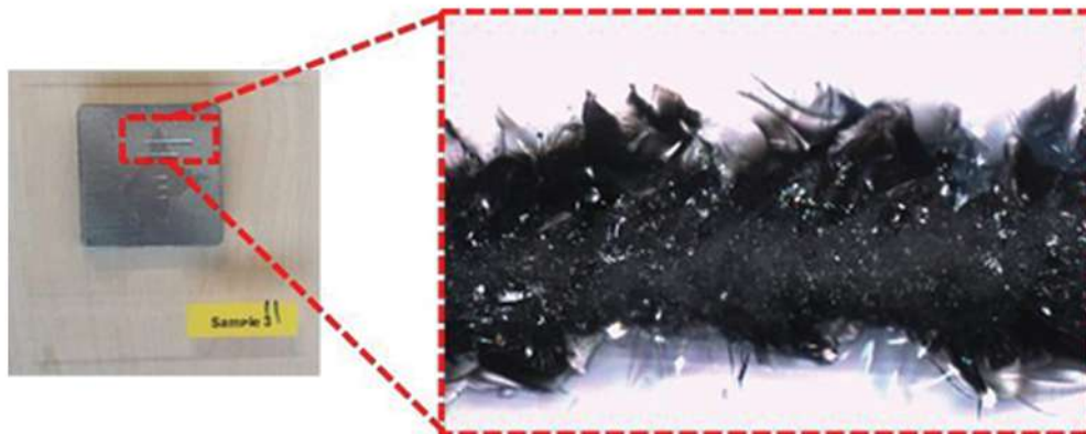
Multiple scratches on the glass specimen
