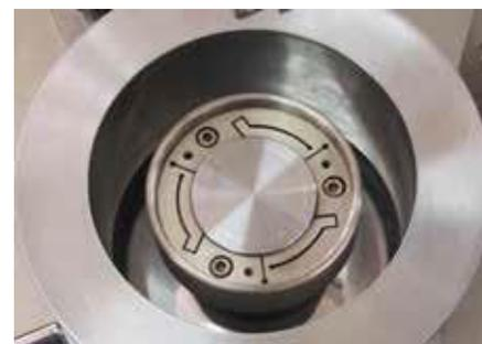
Rotary Drive - Vertical mounted on the UniTest together with a sample holder.
